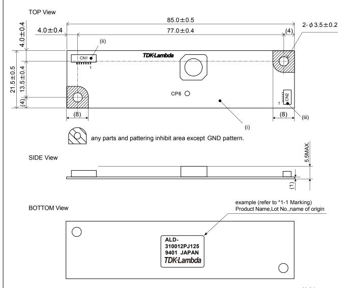
When LED driver is fixing, please confirm screw head and plate form is located within above hatching area include any tolerances.
